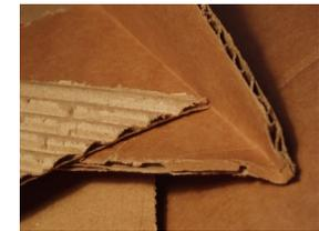
Corrugated cardboard has three layers with two flattened pieces sandwiched around a middle wavy layer.
