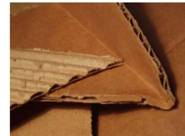
Corrugated cardboard has three layers with two flattened pieces sandwiched around a middle wavy layer.
